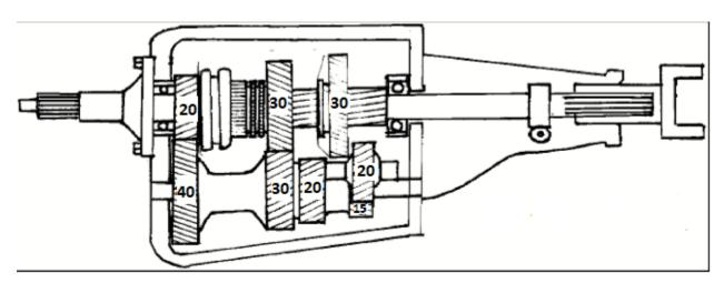
a. What is the gear ratio of the gear above?
