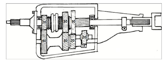
a. What is the gear ratio of the gear above?
