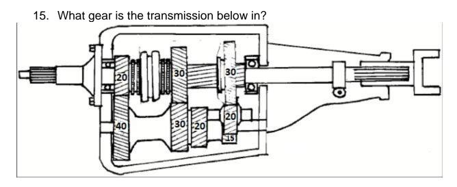
a. What is the gear ratio of the gear above?
